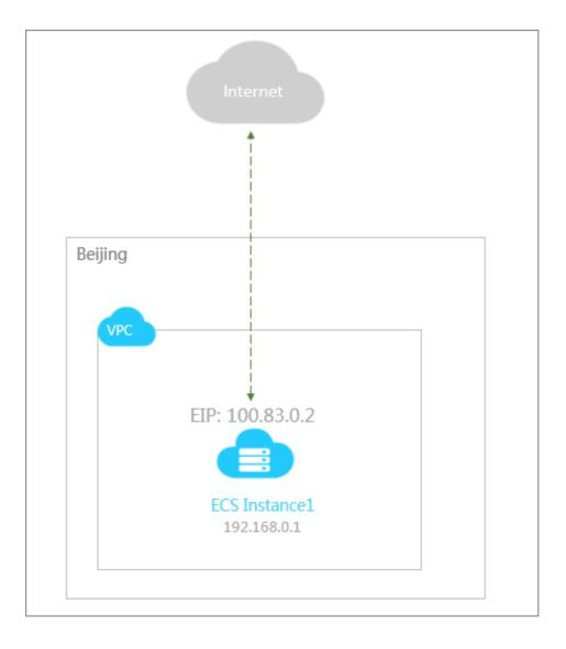
Configure the NAT gateway on the ECS in the VPC to implement communications between the VPC and the Internet. For more information, see Port Mapping and SNAT Configuration.
