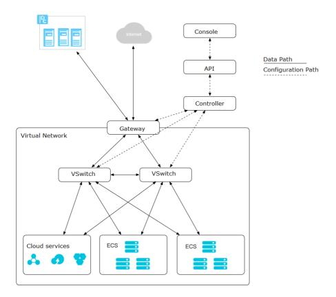
VSwitches and gateways form the key data path. Controllers use the self-developed protocol to forward the forwarding table to the gateway and VSwitches, completing the key configuration path. In the overall architecture, the configuration path and data path are separated from each other.
