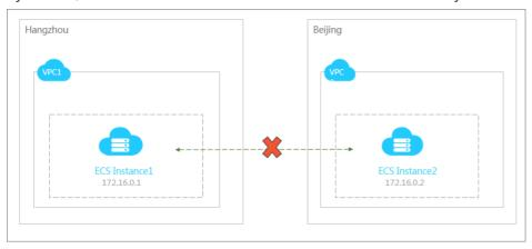
By creating router interfaces on both sides of the VPCs to build a Express Connect on Alibaba's backbone transmission network, you can easily implement fast, secure, reliable, and convenient communications between VPCs. For detailed configurations, see Establish an intranet connection between VPCs in different regions.
