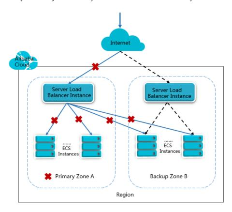
If you add all the ECS instances to the primary zone and have no ECS instances in the backup zone, as shown in the following figure, low latency is achieved at the expense of high availability. In this situation, when the primary zone is unavailable, Server Load Balancer switches to the backup zone. However, there are no ECS instances to handle the distributed requests in the backup zone.
