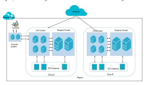
As shown in the following figure, the layer-4 load balancing in each region is actually run in a cluster of multiple LVS machines. The cluster deployment model strengthens the availability, stability, and scalability of the load balancing services in abnormal circumstances.
