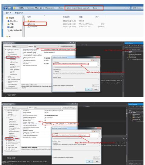
Now the compilation environment has been set up. Click **Build** to compile the executable application, and copy the DLL to the directory of the executable application or to the system directory to run the DLL.
