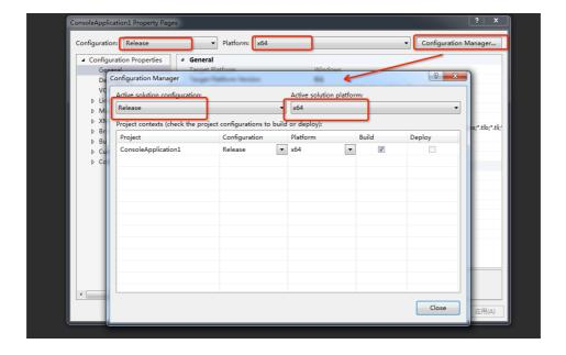
Right-click the project, and choose **Properties** > **Configure Properties** > **General** > **Output Directory**: /**A**. Based on the setting of **Active Solution Platform**, copy all files in the 64-bit lib directory to the output directory /**A**.
