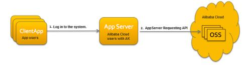
As shown in the figure above, you need to develop an AppServer. Only the AppServer can access the ECS. The ClientApp can read or write data only through the AppServer. The AppServer ensures isolated access to different user data.
