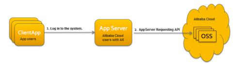
As shown in the figure above, you need to develop an AppServer. Only the AppServer can access the ECS. The ClientApp can read or write data only through the AppServer. The AppServer ensures isolated access to different user data.
