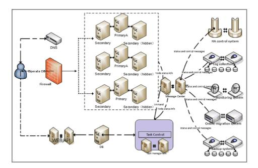
**HA Control System**: Instance high-availability detection modules are used to detect and monitor the operating status of MongoDB instances. If the system determines that the primary node instance is unavailable, it will switch over to the standby node, to ensure the high availability of MongoDB instances.
