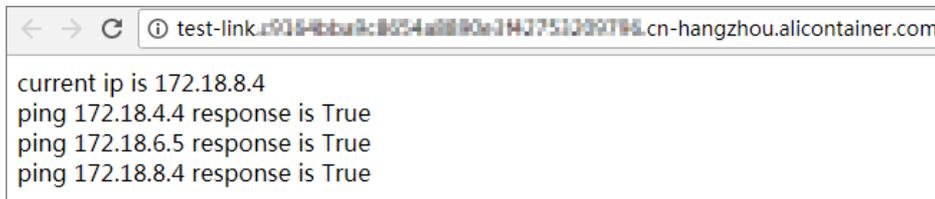
Refresh the page. As shown in the following figure, the container **test-cluster-link\_web\_2** can access the container **test-cluster-link\_web\_1** and container **test-cluster-link\_web\_3**.
