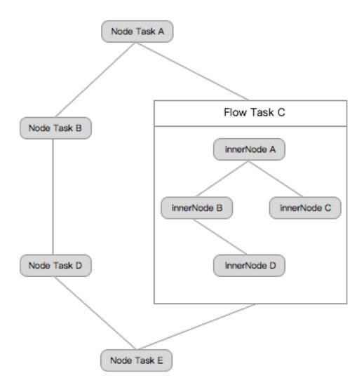
A node task is an operation performed on data. It can be configured to be dependent on other node tasks and flow tasks to form a directed acyclic graph (DAG).
