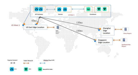
We recommend using the <u>sn1ne family of computing network enhanced instances</u>. This instance type is an enhanced network model, which can meet the architecture's low-latency needs.
